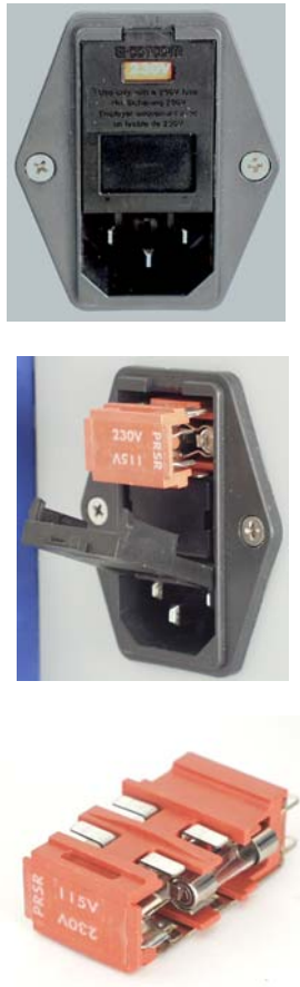
Fig. 4: Fuse location (1 of 2 fuses visible) and line voltage setting
