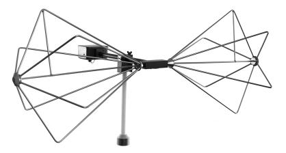
The biconical elements are made from welded aluminum. The elements mount in a balun network fabricated of phenolic and equipped with the necessary impedance-matching components. The lightweight construction provides easy handling and storage.
