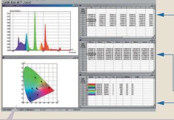
Application software CS-900 for Windows supports Spectroradiometer SR-3AR / SR-UL1R / SR-UL2. You can control SR-3AR / SR-UL1R / SR-UL2 using by the CS-900, and collect, save, plot on a graph and calculate of the measured data and, use them for many purpose.
