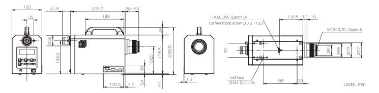
For measuring of Spectral distribution, Luminance, Chromaticity and Correlated color temperature of the light emitted from display device and lamp, SR series Spectroradiometer is suited.
