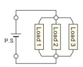
A power supply has no direct branching, but the load is branched using cables.
