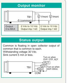
\*Please use TB1 in floating as TB1 and minus output is connected in the internal part.
