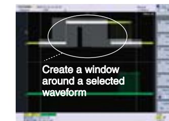
Waveform window search Select a waveform in History Memory and create a window around the waveform by moving up/down/left/right from the waveform. Search for waveforms that fall inside or outside the window.
