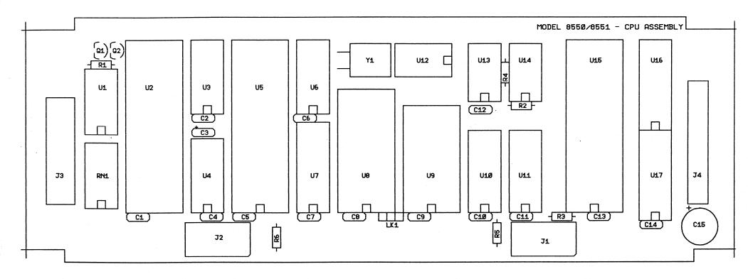
Figure 9-5. CPU Board - Components Location
