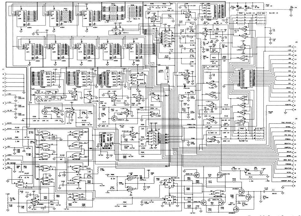
Figure 9-8. Current Generator Board
