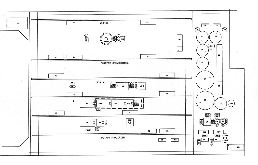
Figure 9-3. Main Board - Components Location
