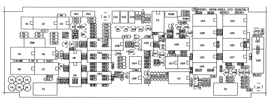
Figure 9-11. VCO Board - Components Location
