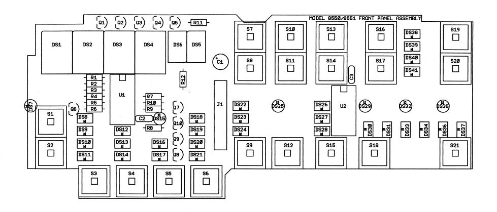
Figure 9-7. Keyboard and Display - Components Location
