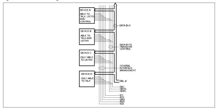
Any given system can have only one controller (control may be passed to an appropriate device through a special command). Any number of talkers or listeners may be present up to the hardware constraints of the bus. The bus is limited to 15 devices, but this number may be reduced if higher than normal data transfer rates are required or if long interconnect cables are used.
