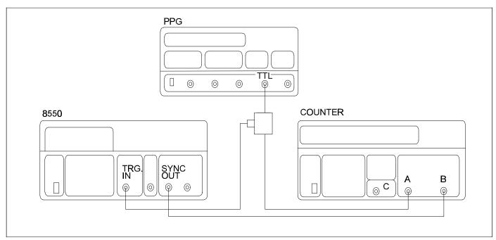
Figure 5-1. PLL Phase Offset Accuracy Check.
