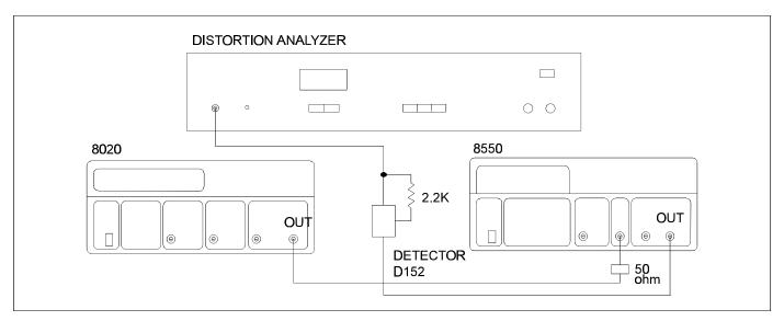
Figure 5-3. Amplitude Modulation Operation Check
