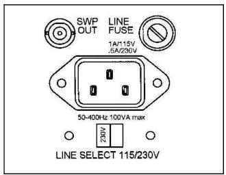
Figure 2-1. Line Voltage and Fuse Holder.
