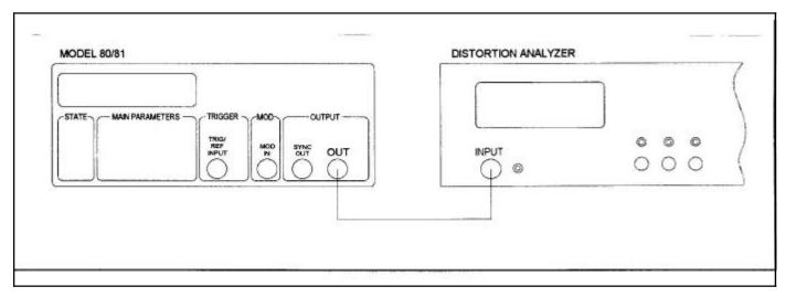
Figure 7-1. Connection - Distortion Adjustment.
