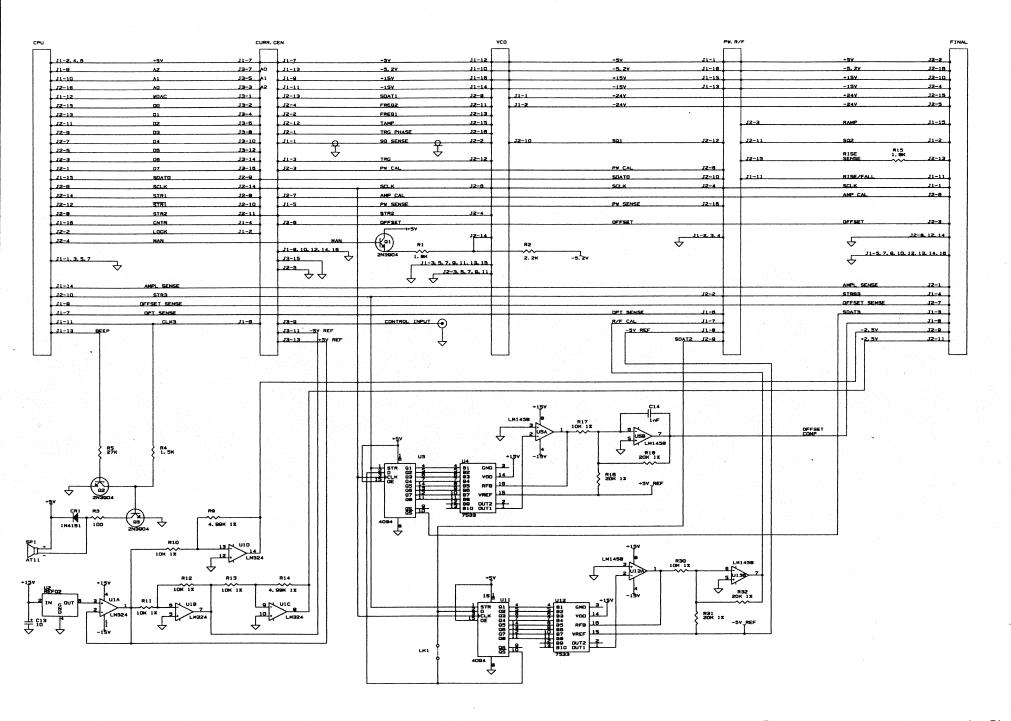
Figure 9-2. Main Board - Inter-connection Diagram
