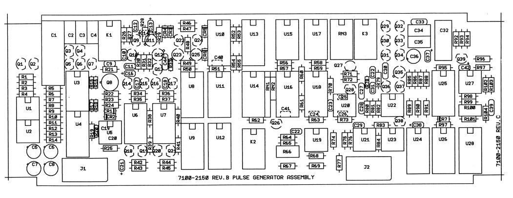
Figure 9-15. Pulse Generator Board - Components Locatic
