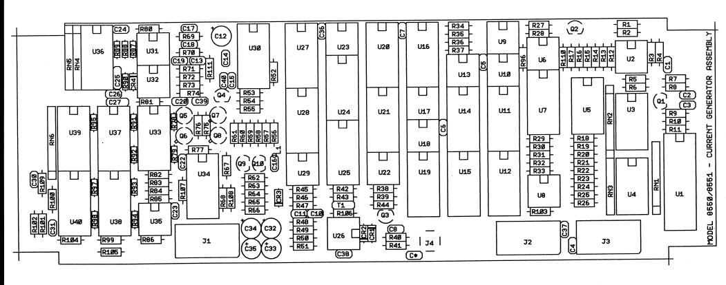
Figure 9-9. Current Generator Board - Components Location
