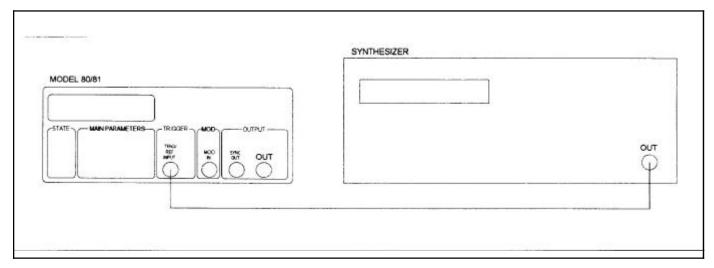
Figure 7-5. Connection - Reference Oscillator Adjustment.
