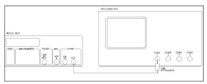
Figure 7-3. Connection - Squarewave Response Adjustment.
