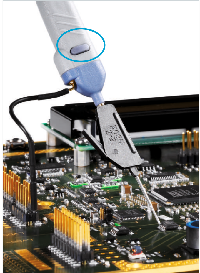
Practical design: micro button for convenient instrument control. Diverse probe tips and ground cables are included as standard accessories.
